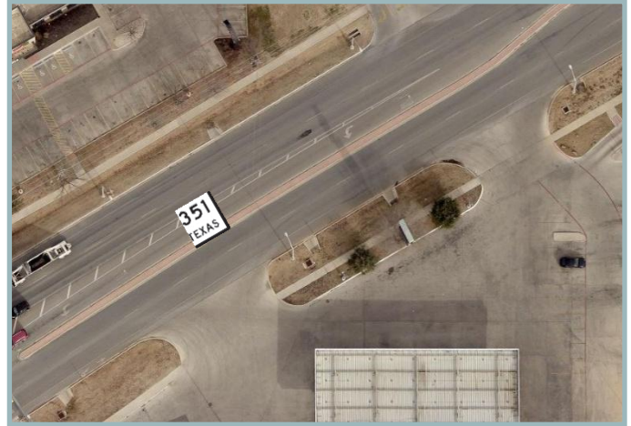
Figure 2.20. Sidewalk interrupted at wide driveways. Image credit: 2022 Pictometry City of Abilene GIS Department, accessed September 26, 2024.
